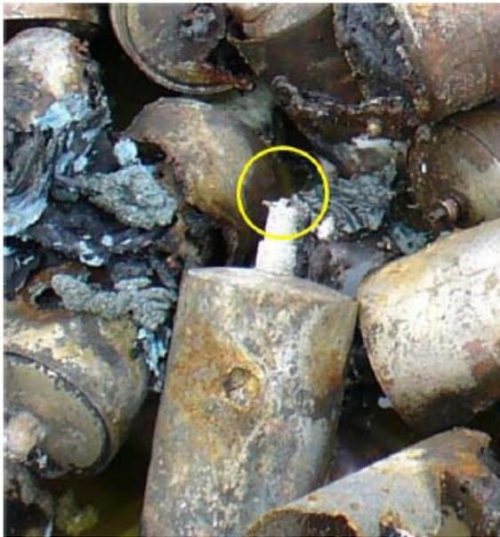
Photo, from Chemical Safety Board Report showing an oxygen generator with activation pin circled, in EQ rubble
