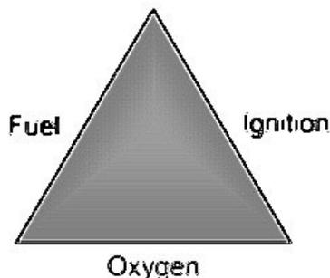
For a fire to occur, all three elements (a fuel, oxygen, and an ignition source) must be present. The oxygen can come from the air, which is composed of 21% oxygen. In a few situations, the oxygen can come from a chemical that is in contact with the fuel, for example nitrates and ethers. The ignition source could be static electricity, lightning, another fire, a lighted cigarette, or sparks from equipment. The fuel is anything that will burn.
